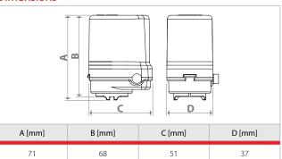
THERMO-ELECTRIC ACTUATORS NORMALLY CLOSED R473, R473M
