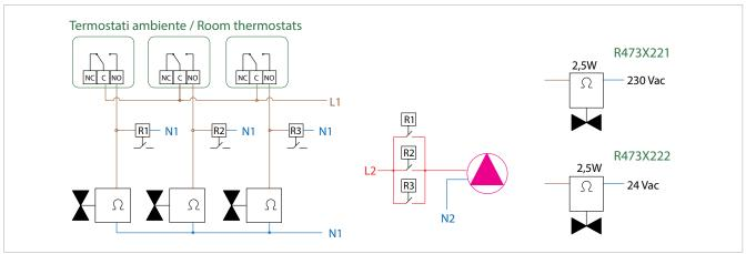
**R473M** thermo-electric actuators equipped with a stroke-end micro switch enable to easily activate circulators or zone valves. They are generally connected to ambient thermostats taking into consideration that the R473M is closed when there is no voltage (while the micro switch is electrically open in such status). To control significant power loads, we recommend installing a relay to prevent overloading of the actuator micro switches.
